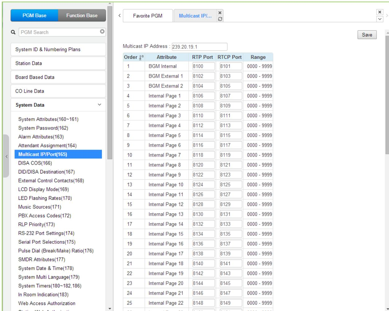
**Figure 4.4.5.5-1 Multi-cast IP/Port**
