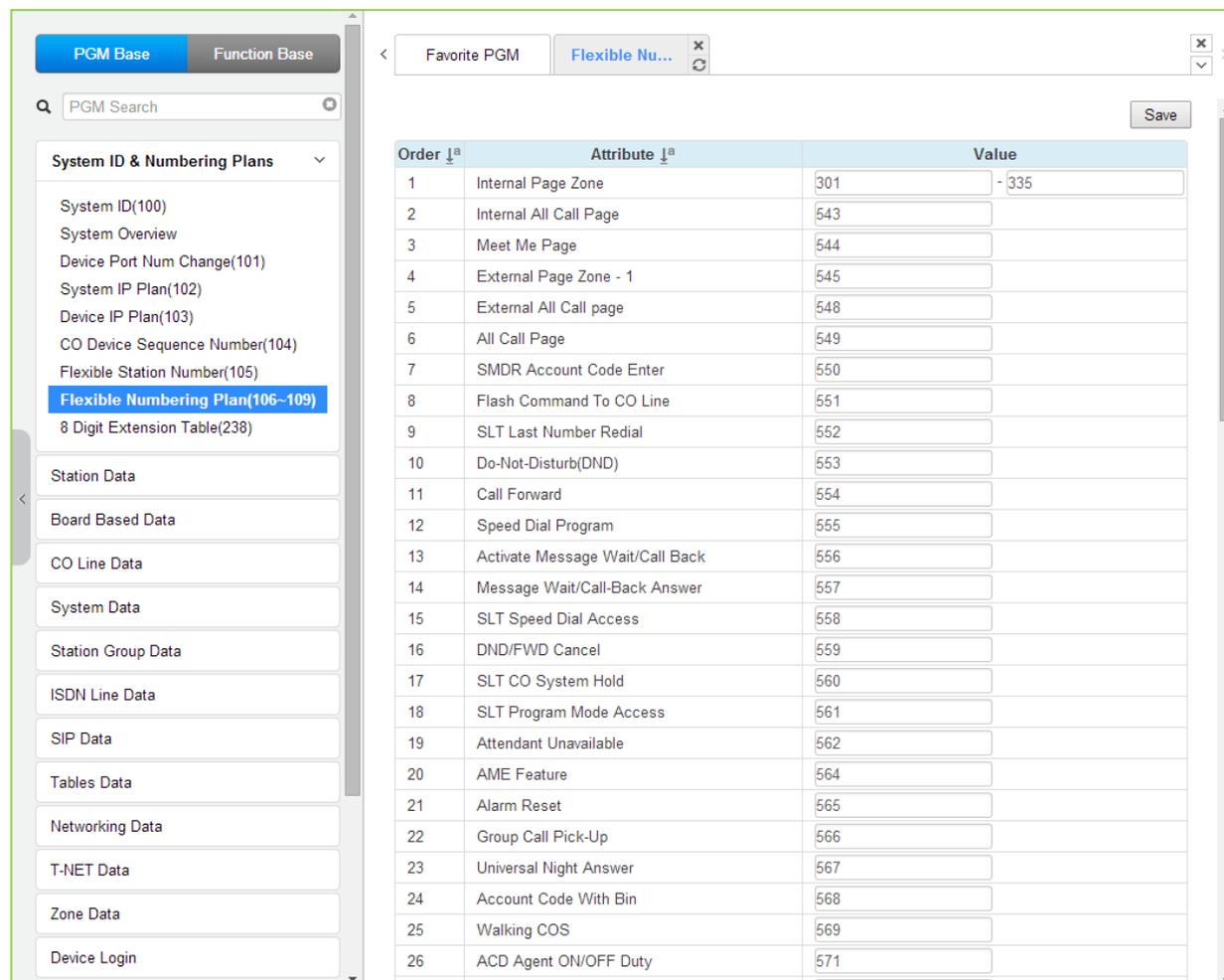
Figure 4.4.1.8-1 Flexible Number Plan
