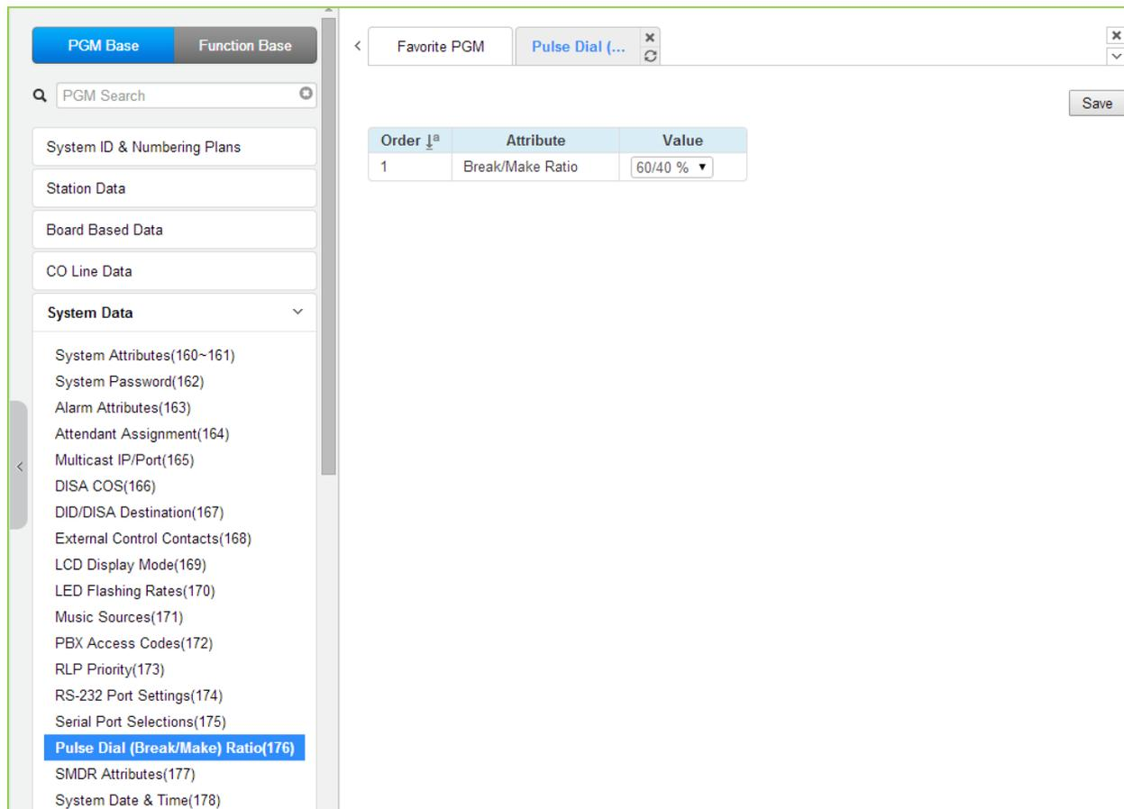
Figure 4.4.5.16-1 Break/Make Ratio
