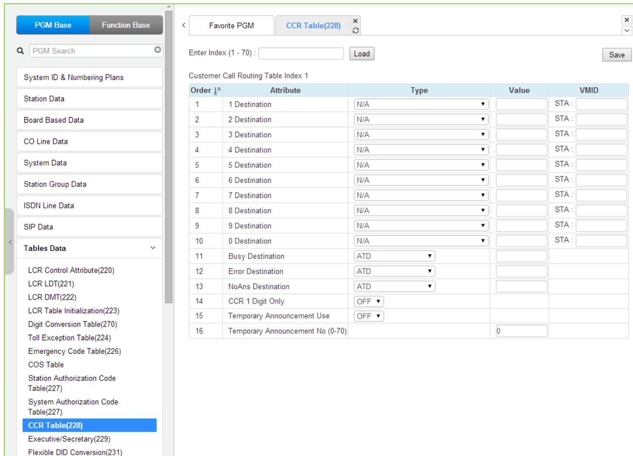
**Figure 4.4.9.10-1 Customer Call Routing Table**
