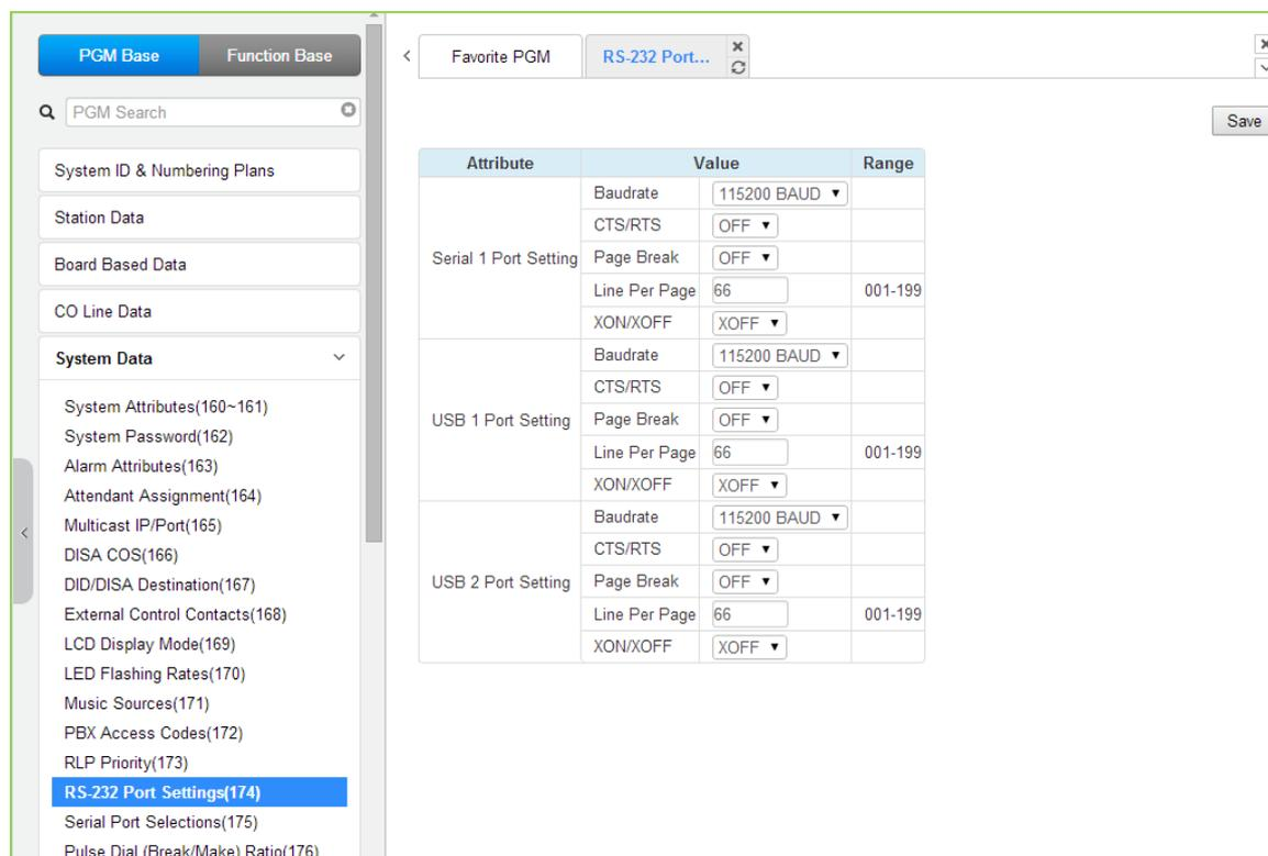
Figure 4.4.5.14-1 RS232 Port and USB 1&2 port Settings
